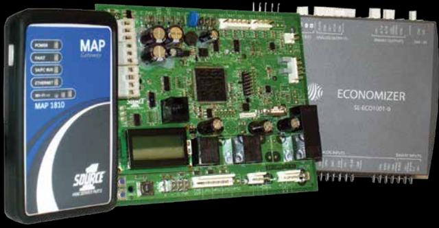
Integrated by design: The Simplicity® SE platform incorporates functionality for motors, drives, actuators and different controllers all on one board.
